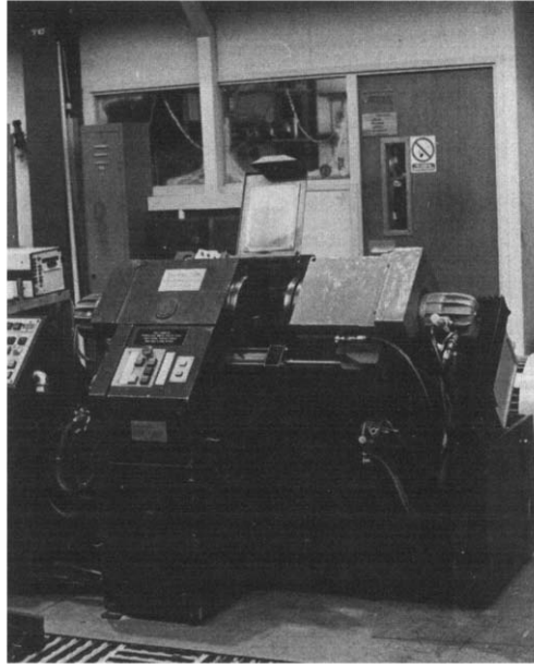
Fig. 1. Model FW7 continuous drive, orbital friction welding machine (total height about 1.5 m). Drive spindles can be seen at the top centre of the machine, below uplifted protection shield. Controls and computer print-out are at extreme left.
